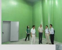
Photo 7: Reverberation room for testing acoustic panels
