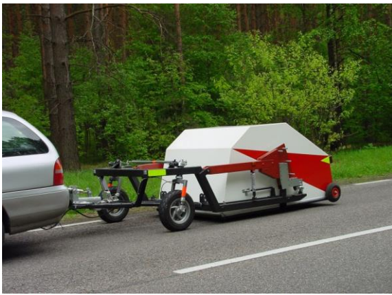
Trailer "Tiresonic Mk4" for tyre/road noise measurements
