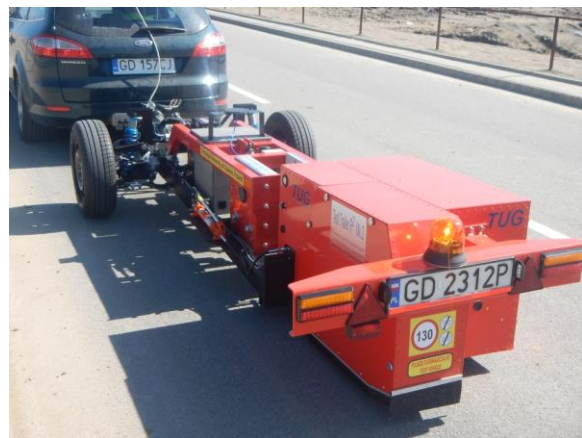
Trailer R 2 Mk.2 for tyre rolling resistance measurements
