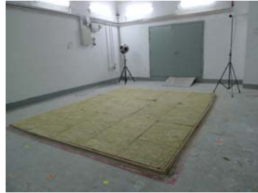
Laboratory Sound Absorption Tests
