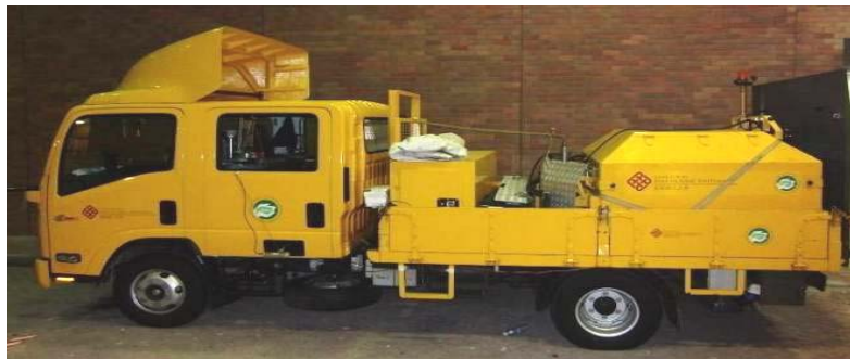
Figure 4: Setup of the on-road test with the CPX trailer fixed onto the deck of the light goods vehicle
