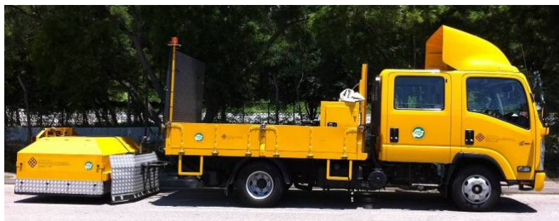
Figure 1: Overview of CPX tyre/road noise measurement
