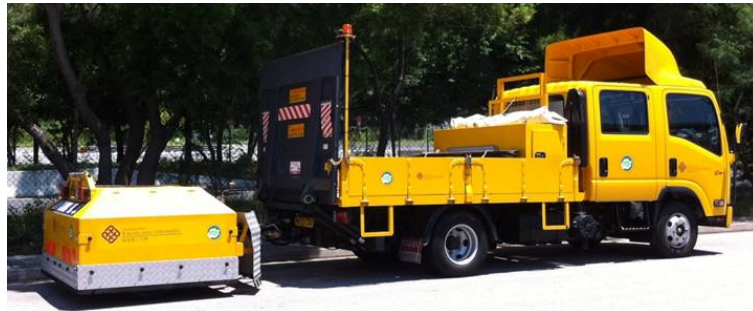
Figure 1: Overview of the CPX tyre/road noise measurement system
